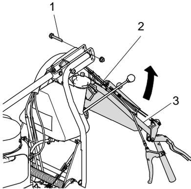
1. Slacken the screw for the height adjustment of the handlebar (1) and pull it out sideways.
