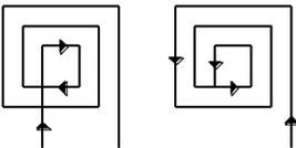
To avoid blockage during the ejection of grass, we recommend, for flat terrain, to proceed according to the mowing patterns. Mulch is shredded into much smaller pieces when you mow the terrain once again in the opposite direction.
