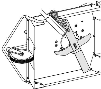
After each use, you should clean the device thoroughly, especially the bottom side and the blade.
